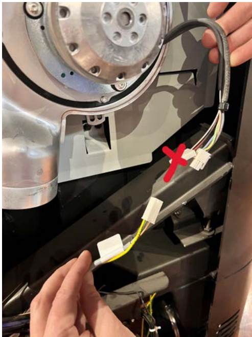
Fig. 48: Connecting the cables
