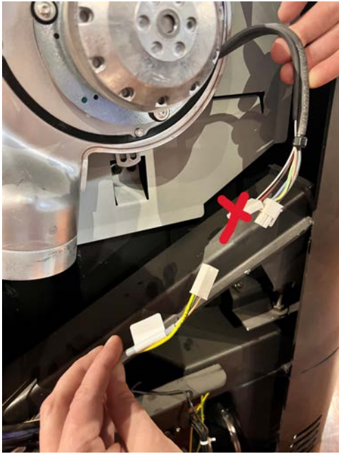
Fig. 9: Connecting the cables
