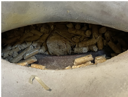
Fig. 19: Fire lighter below pile of pellets
