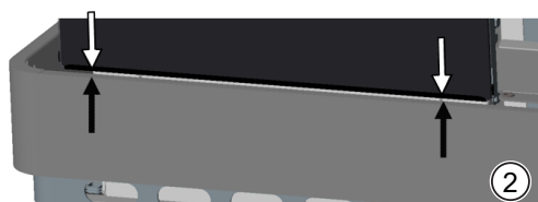
Fig. 15: Aligning the cladding base
