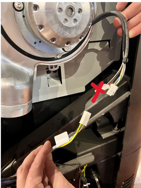
Fig. 74: Connecting the cables
