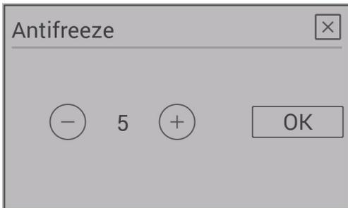
The anti-frost menu is used to automatically start the stove at a specified temperature. The menu only functions when the timer function is enabled (set in the timer menu).
