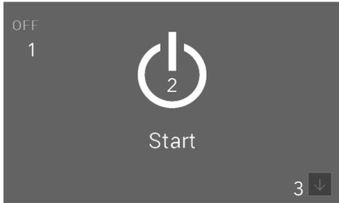
The stove is started or stopped by pressing the start / stop button for longer than 2 seconds.
