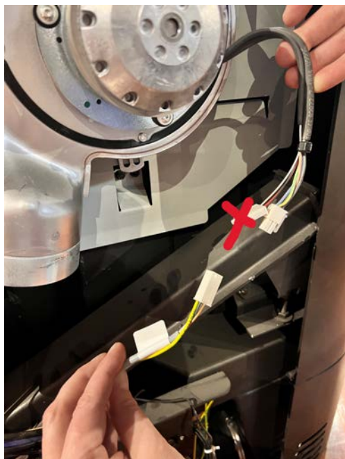
Fig. 23: Connecting the cables
