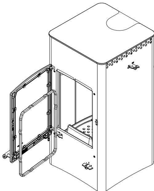
Fig. 20: Remplacer le joint
