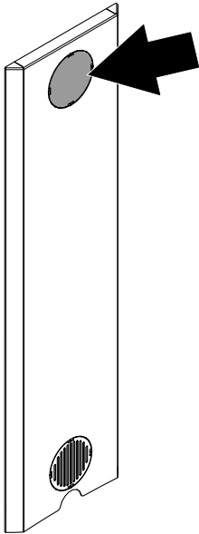
Fig. 9: Removing the perforated cut-out
