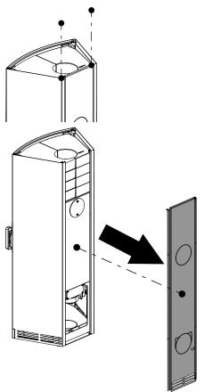
Fig. 34: Undoing the screws from the rear
