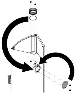
Fig. 12: Replacing cover and bracket
