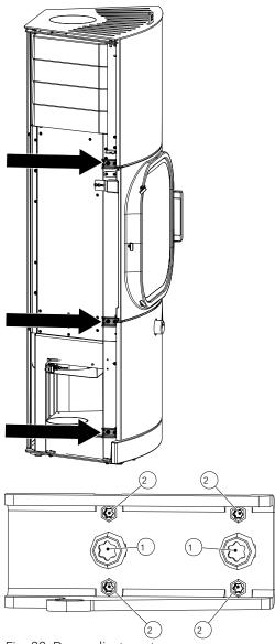
Fig. 22: Door adjustment screws
