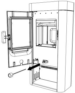
Fig. 16: Remove rotary control unit
