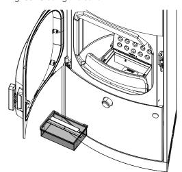
Fig. 31: Removing and emptying the ash box
