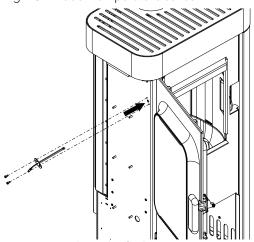
Fig. 19: Attaching the firebox temperature sensor
