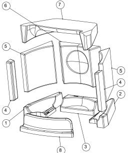
Fig. 15: Mounting the Keramott
