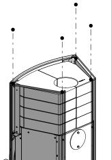
Fig. 35: Detaching the side cladding
