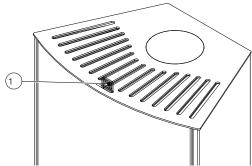
Fig. 32: Convection air control
