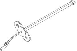
Fig. 18: Firebox temperature sensor
