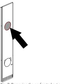
Fig. 9: Removing the perforated cut-out
