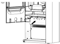
Fig. 21: Mounting the cover
