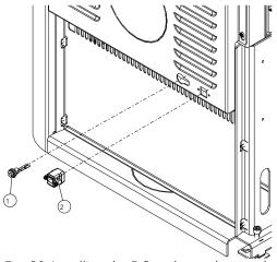
Fig. 20: Installing the DC socket and network socket
