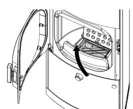
Fig. 29: Putting the cover on the ash box
