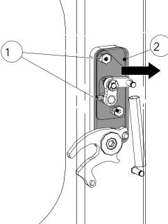
Fig. 24: Adjusting the door lock
