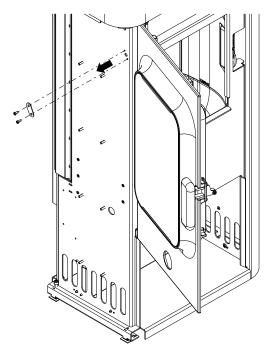
Fig. 17: Removing the cover plate
