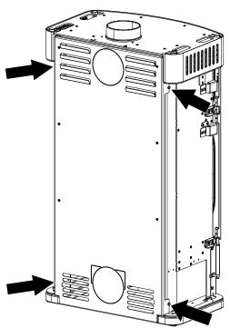
Fig. 50: Undoing the screws on the left and right of the rear panel
