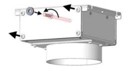
1) Insert the 125 mm hexagon rod supplied into the air box and turn fully counterclockwise.
