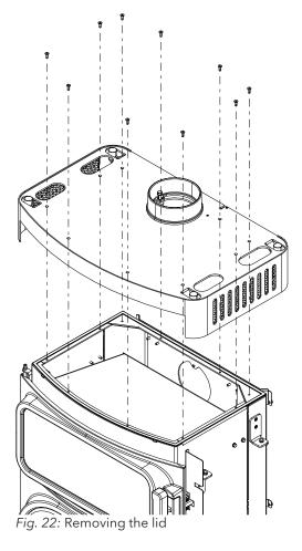
3) Undo all the screws from the lid and remove the lid.
