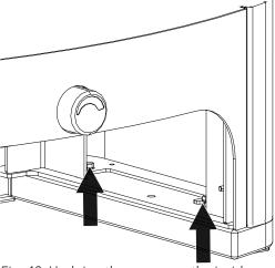
Fig. 48: Undoing the screws on the inside
