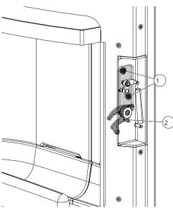
Fig. 38: Adjusting the door lock
