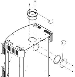
Fig. 13: Remove cover and bracket
