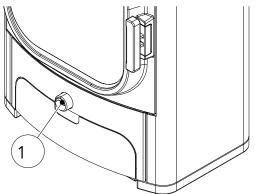
Fig. 39: Primary/secondary air controller
