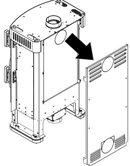
Fig. 51: Detaching the rear panel
