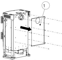
Fig. 21: Removing the radiation protection
