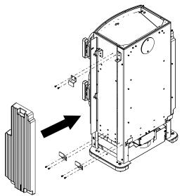
Fig. 23: Mounting HMS holder and HMS brick
