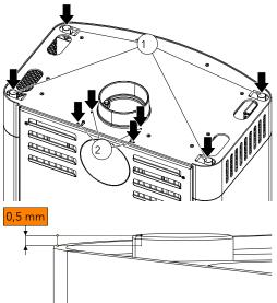
Fig. 7: Adjusting the rubber cushions
