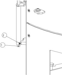
Fig. 37: Adjusting the closing pressure of the door
