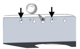
Fig. 34: Mounting the cover
