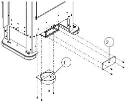
Fig. 27: Removing the supply air flange
