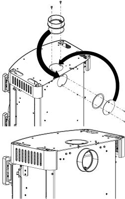
Fig. 14: Replacing cover and bracket
