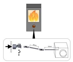
Fig. 30: Remove rotary control unit
