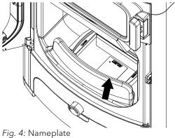
The type plate is located in the firebox below the ash box.
