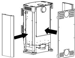
Fig. 19: Mounting the rear panel and side cladding
