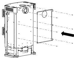
Fig. 18: Mounting the radiation protection
