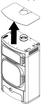
Fig. 10: Removing the hob
