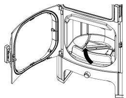
Fig. 44: Putting the cover on the ash box
