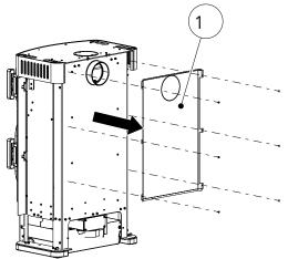
Fig. 12: Removing the radiation protection
