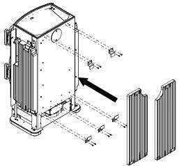
Fig. 24: Mounting HMS brick at the rear
