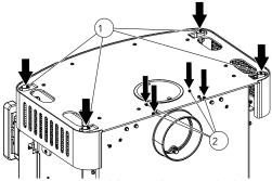
Fig. 15: Setting rubber cushions and adjusting screws
