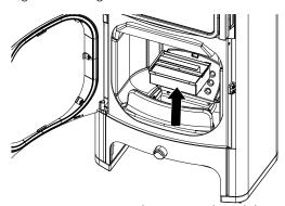
Fig. 46: Removing and emptying the ash box
