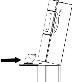
Fig. 46: Tilting the stove on the base
