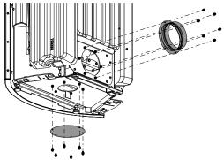
Fig. 24: Removing bracket and cover
