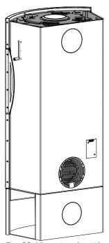
Fig. 22: Mounting the side cladding
