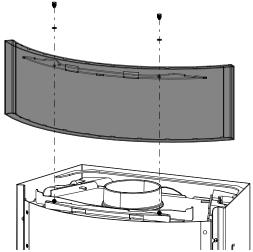
Fig. 30: Attaching and fastening the trim
