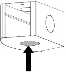
Fig. 23: Removing the perforated cut-out
