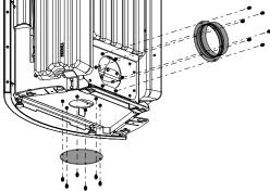
Fig. 19: Removing bracket and cover
