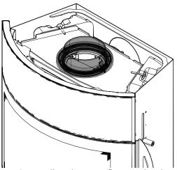
Fig. 35: Installing the rotary flue pipe bracket
