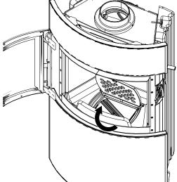
Fig. 66: Placing and engaging lid on ash box
