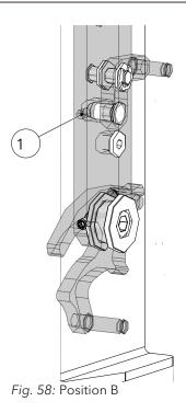
4) The closing force can be adjusted by loosening or tightening the threaded bolt (1).
