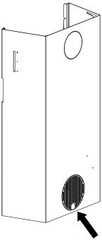
Fig. 13: Removing the perforated cut-out
