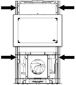
4) Loosen the marked screws left and right.
