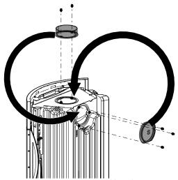
Fig. 10: Replacing cover and bracket
