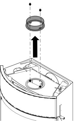
Fig. 44: Removing the flue pipe bracket
