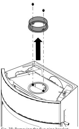
Fig. 38: Removing the flue pipe bracket
