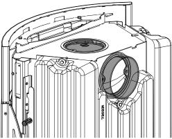
Fig. 11: Cover and bracket replaced
