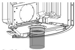
Fig. 17: Fastening the pipe
