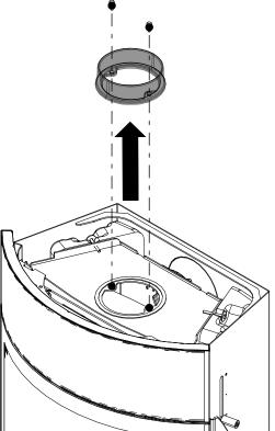
Fig. 34: Removing the flue pipe bracket
