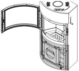
Fig. 32: Inserting the trim at the bottom
