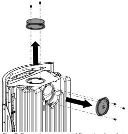
Fig. 9: Removing cover and flue pipe bracket
