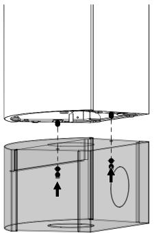
Fig. 49: Fitting the base from below
