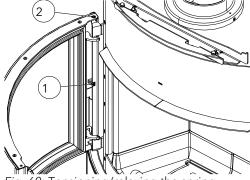
Fig. 60: Tensioning/relaxing the spring
