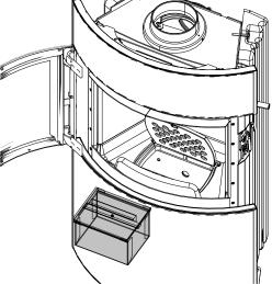
Fig. 67: Removing and emptying the ash box
