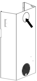
Fig. 8: Removing the perforated cut-out
