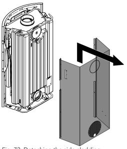
Fig. 72: Detaching the side cladding
