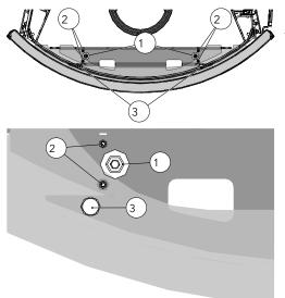
Fig. 51: Adjusting the trim at the top
