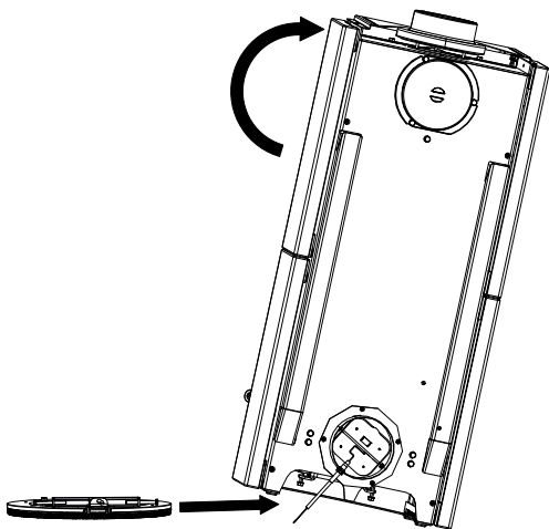
Fig. 21: Tilting the stove sideways
