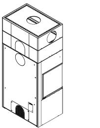
Fig. 22: Extension boxes on HMS bricks
