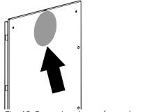
Fig. 13: Removing the perforated cut-out
