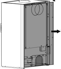
Fig. 40: Unhinging the rear panel
