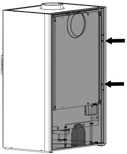
1) Undo screws via the slots.
