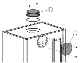
Fig. 14: Remove cover and bracket
