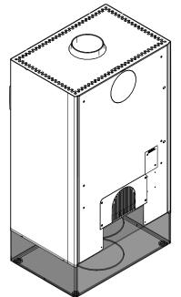
Fig. 18: Placing the stove on to the base
