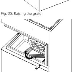
Fig. 36: Putting the cover on the ash box
