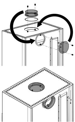
Fig. 15: Replacing the cover and bracket
