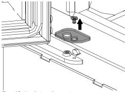
Fig. 42: Undoing the spring cover
