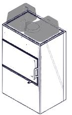
Fig. 20: Installing the HMS bricks
