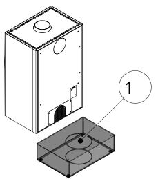
Fig. 17: Base with cut-out
