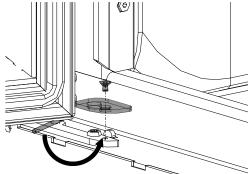
Fig. 26: Hanging the door and tightening the spring
