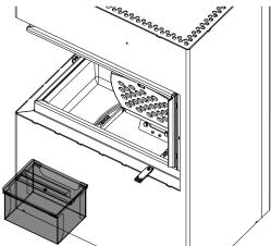
Fig. 38: Removing and emptying the ash box
