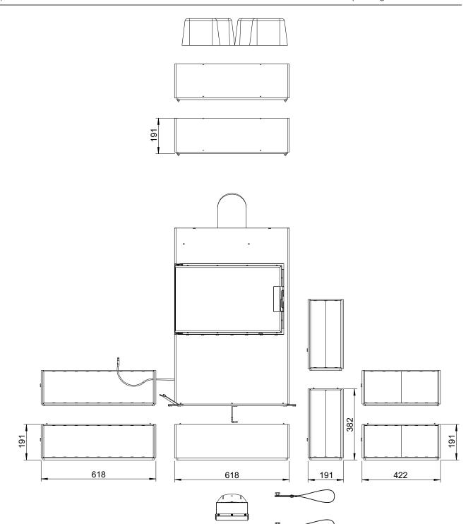
Fig. 2: Dexter I & r set-up box dimensions
