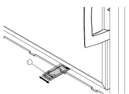
Fig. 31: Primary- secondary air damper
