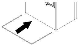
Fig. 9: Inserting the shadow gap
