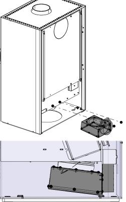
Fig. 11: Installing the supply air adapter
