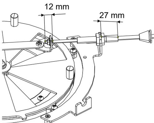
Fig. 52: Raccorder le câble Bowden
