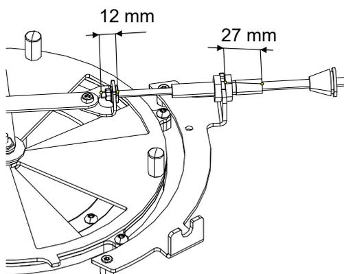
Fig. 57: Raccorder le câble Bowden
