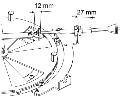
Fig. 50: Raccorder le câble Bowden
