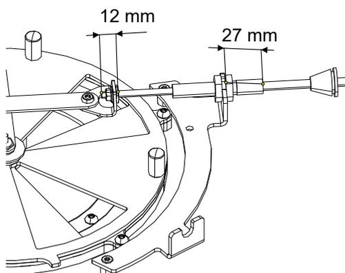
Fig. 49: Raccorder le câble Bowden
