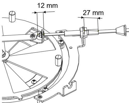
Fig. 63: Raccorder le câble Bowden
