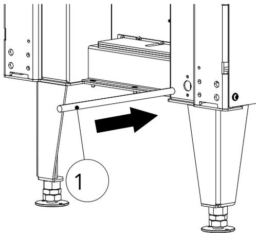
Fig. 62: Enfiler le câble Bowden
