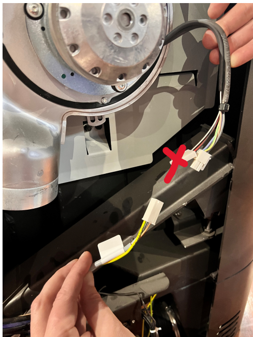
Fig. 23: Connecting the cables
