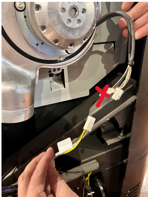
Fig. 80: Connecting the cables
