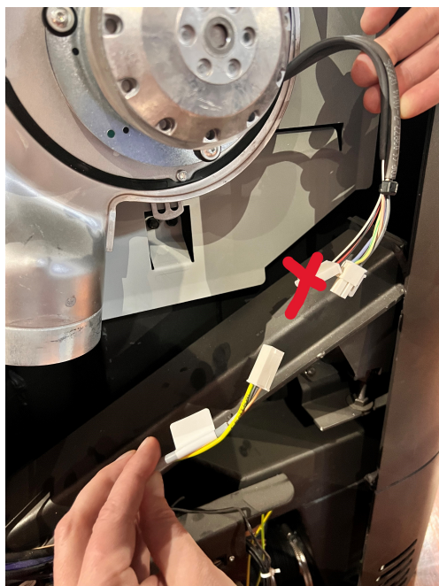
Fig. 9: Connecting the cables
