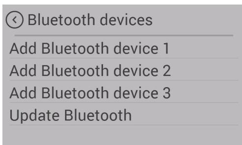
The SMART SPOT wireless room thermostat is an available to you as an option for your pellet stove. SMART SPOT works via Bluetooth technology. When used it must be enabled once with this menu item.
