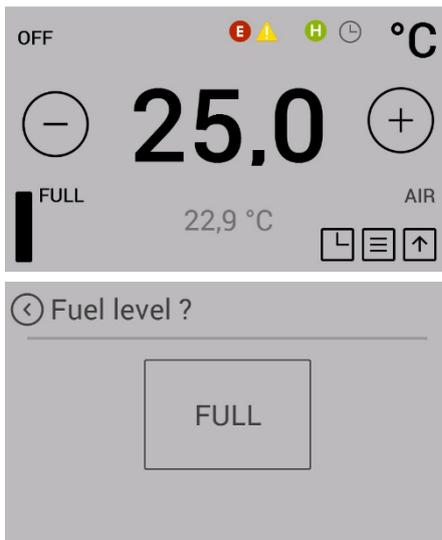
The filling level indicator keeps you informed of the filling level of your pellet hopper. If the filling level falls below a certain level, a warning is shown on the display. Each time that the hopper is filled, the filling level must be manually updated.
