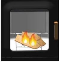
Upon elapse of the 'Hybrid start' the furnace switches to this operating phase. Here it is ensured that all pellets combust in the combustion bowl and that the firewood continues to be inflamed.
