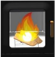
In this operating status, the riddling grate is opened after approx. 2 minutes. As a result, the primary air damper is closed and the firewood continues to be fanned until a certain temperature in the firebox is reached (depending on the selected heat output). Once this temperature has been obtained, the stove switches to the status "Firewood mode".
