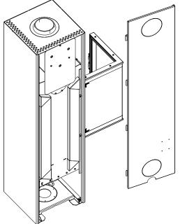
Fig. 53: Removing the rear panel
