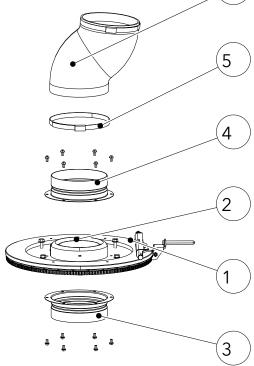
Fig. 35: Turntable with connecting parts
