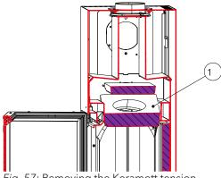
Fig. 57: Removing the Keramott tension plate
