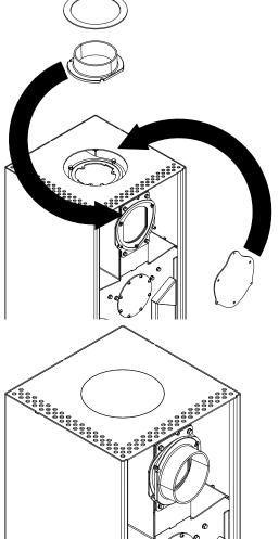
Fig. 12: Replacing the cover and bracket
