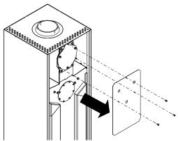
Fig. 21: Dismantling the heat shield
