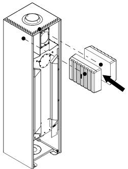
Fig. 23: Inserting the HMS stones
