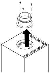
Fig. 26: Removing the flue pipe bracket
