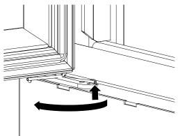
Fig. 55: Releasing the spring
