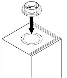
Fig. 33: Fitting the swivel elbow coupling
