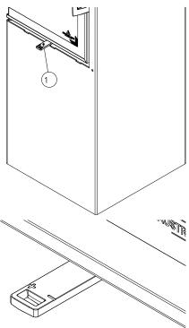
1) Open (+) and closed (-) (primary/secondary air controller)
