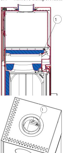
Fig. 7: Remove transport fastenings
