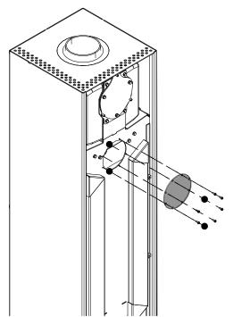
Fig. 44: Remove inspection cover
