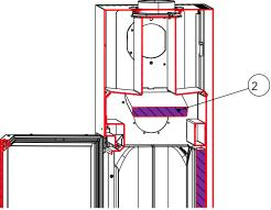
Fig. 58: Taking out the Keramott deflection
