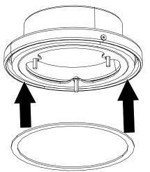
Fig. 32: Attaching the seal to swivel elbow coupling
