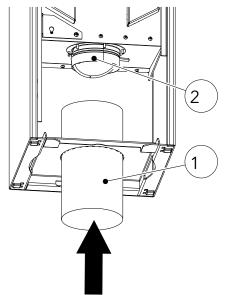
Fig. 18: Inserting the pipe
