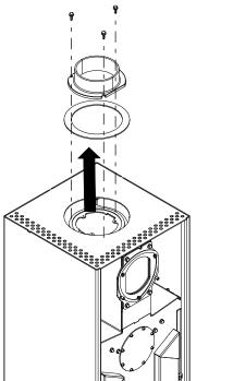
Fig. 11: Removing the bracket with seal
