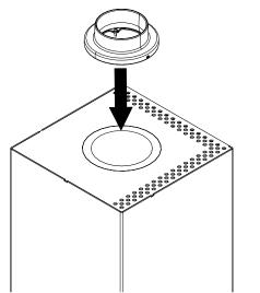
Fig. 28: Fitting the swivel elbow coupling
