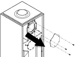
Fig. 10: Removing the rear flue pipe cover
