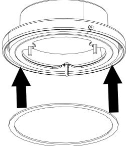
Fig. 27: Attaching the seal to swivel elbow coupling
