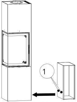
Fig. 25: Mounting the side box
