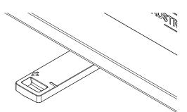
Fig. 40: Primary/secondary air controller
