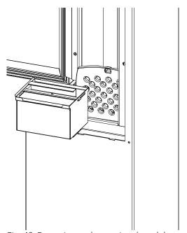
Fig. 49: Removing and emptying the ash box
