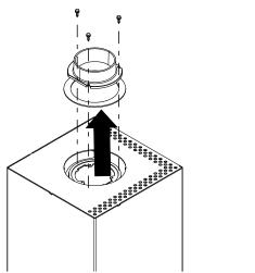
Fig. 31: Removing the flue pipe bracket
