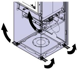
Fig. 6: Removing the transport lock
