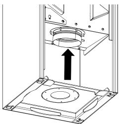
Fig. 15: Mounting the external air connection at the rear
