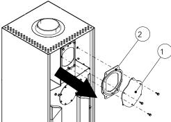
Fig. 22: Removing the rear flue pipe cover
