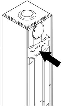
Fig. 45: Vacuum flue gas passages
