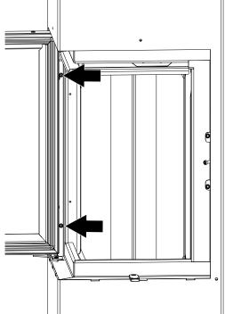
Fig. 51: Removing the screws from the rear panel
