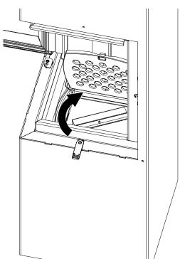
Fig. 47: Putting the cover on the ash box
