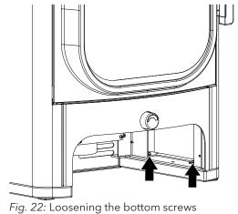
3) Loosen screws on the inside on the right.
