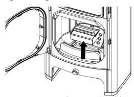
Fig. 56: Removing and emptying the ash box
