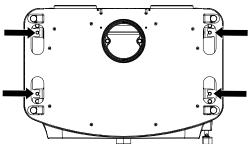
Fig. 57: Undoing the screws from above
