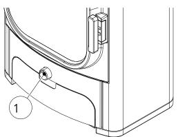
Fig. 49: Primary/secondary air controller
