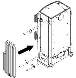
Fig. 34: Mounting HMS holder and HMS brick
