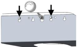
Fig. 45: Mounting the cover
