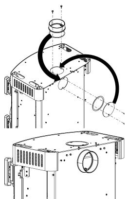
Fig. 14: Replacing cover and bracket
