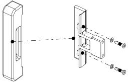
Fig. 26: Mounting the wooden handle
