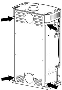
Fig. 60: Undoing the screws on the left and right of the rear panel
