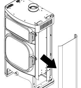
Fig. 23: Detaching the right-hand side cladding
