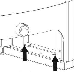
Fig. 58: Undoing the screws on the inside
