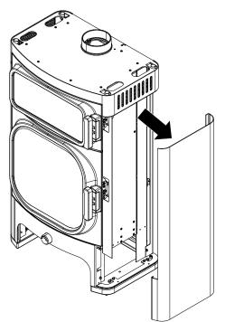
Fig. 59: Detaching the side cladding
