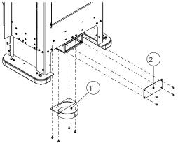
Fig. 38: Removing the supply air flange
