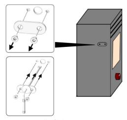
Fig. 42: Fixing the firebox temperature sensor
