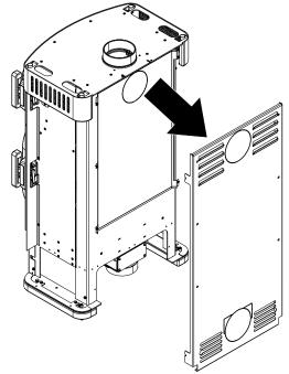
Fig. 61: Detaching the rear panel
