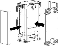
Fig. 19: Mounting the rear panel and side cladding
