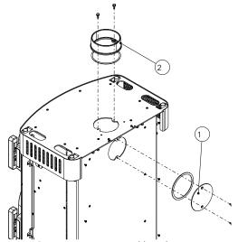
Fig. 13: Remove cover and bracket
