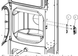
Fig. 28: Mounting adapter plate and catch
