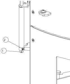
Fig. 48: Adjusting the closing pressure of the door
