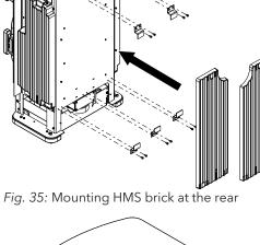
7) Mount the HMS holders as shown on the rear of the stove and attach the HMS bricks to the holders.
