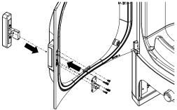
Fig. 27: Mounting the new door handle
