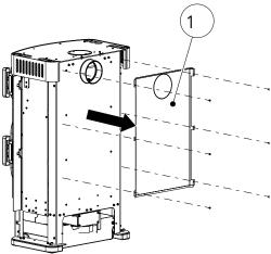
Fig. 12: Removing the radiation protection
