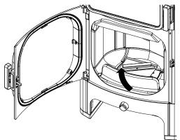
Fig. 54: Putting the cover on the ash box
