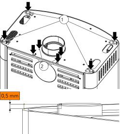
Fig. 7: Adjusting the rubber cushions
