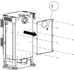
Fig. 32: Removing the radiation protection
