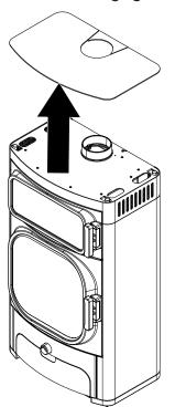
Fig. 10: Removing the hob
