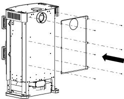
Fig. 18: Mounting the radiation protection
