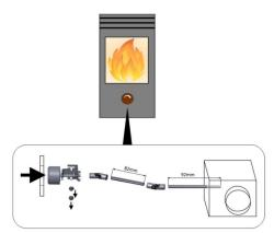
Fig. 41: Remove rotary control unit
